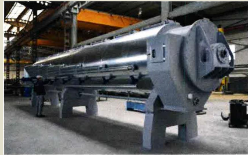
Radiant Heat Processor Sub-system
